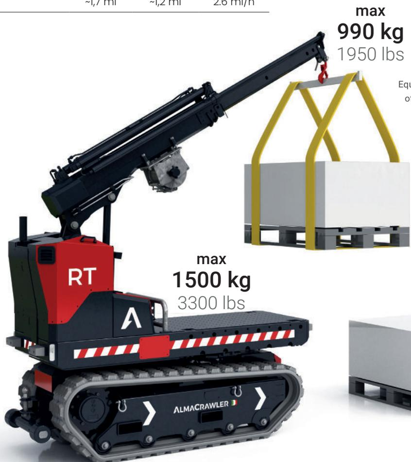
Equipped with a telescopic crane, it has a maximum lifting capacity of 990 kg - 1950 lbs and a variable outreach that can be used on slopes up to +/-10° longitudinal and +/- 5° lateral. The M-Crane 1030 RT, with a maximum capacity of 1500 kg - 3300 lbs, can handle a wide range of loads, making it a versatile solution for a variety of material handling needs.
