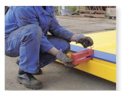
Fit the plates with the lower limit pins. Put on the rolling struts, push them against the limit pins and fix them with the upper limit pins.
