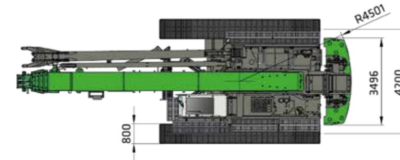
**i** **Weight:** approx. 56.1 t (2 winches, 15 m fly jib, 50 t hook, without crawler tracks, without platform)
