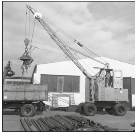
1962: rope-driven S833 with elevated operator cab
